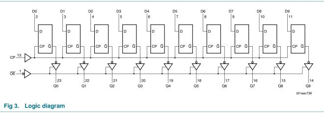
10-bit D-type flip-flop; positive-edge trigger; 3-state
